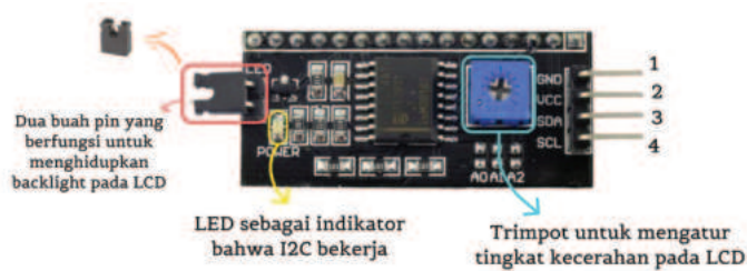
Gambar 9.21 Pin Modul I2C
